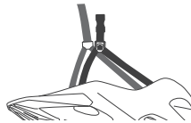
7 Left Temple Straps and Right Temple Straps Have Matching Lengths
